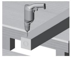
8. Be sure to drill into the steel pipe. This process will provide you with additional clearance to permit you to insert and push the <sup>3</sup>/<sub>8</sub>" diameter bolt completely through the PermaPost<sup>®</sup> and the vertical legs of the bracket. Test fit the mounting brackets at the top and bottom of the PermaPost<sup>®</sup> to ensure that you can push the bolt completely through.
