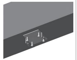
11. Attach the second bracket to the floor. If the floor surface is wood, pre-drill <sup>1</sup>/<sub>8</sub>" diameter holes and use (4) <sup>1</sup>/<sub>4</sub>"x 1<sup>1</sup>/<sub>2</sub>" screws. If the floor surface is concrete, drill 3/16" diameter holes and use (4) <sup>1</sup>/<sub>4</sub>"x 3<sup>1</sup>/<sub>4</sub>" concrete screws. BE SURE THE BEAM BRACKET AND FLOOR BRACKET ARE FACING THE SAME DIRECTION.
