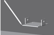
10. The 4 holes in the bottom of each mounting bracket will receive the mounting screws. Pre-drill 1/8" diameter holes and attach one bracket to the beam using (4) 1/4"x 11/2" screws.
