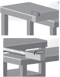
5. Take one mounting bracket and slide it over the bottom of the PermaPost<sup>®</sup>. Position the bottom plate of the bracket so it is aligned evenly with the bottom of the PermaPost<sup>®</sup>.
