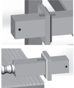
13. Slide the PermaPost<sup>®</sup> into the brackets you just mounted. Align the holes that you drilled through the PermaPost<sup>®</sup> in step 6 with the holes in the vertical legs of the mounting brackets.
