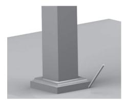
b. Use a tube of clear, water-based construction adhesive in a caulk gun, and place a thick bead of adhesive on the pencil line you traced around the base trim ring. Slide the base trim ring down into place and push it firmly into the thick bead of clear construction adhesive. Wipe off excess adhesive with a damp rag and let the adhesive set.
